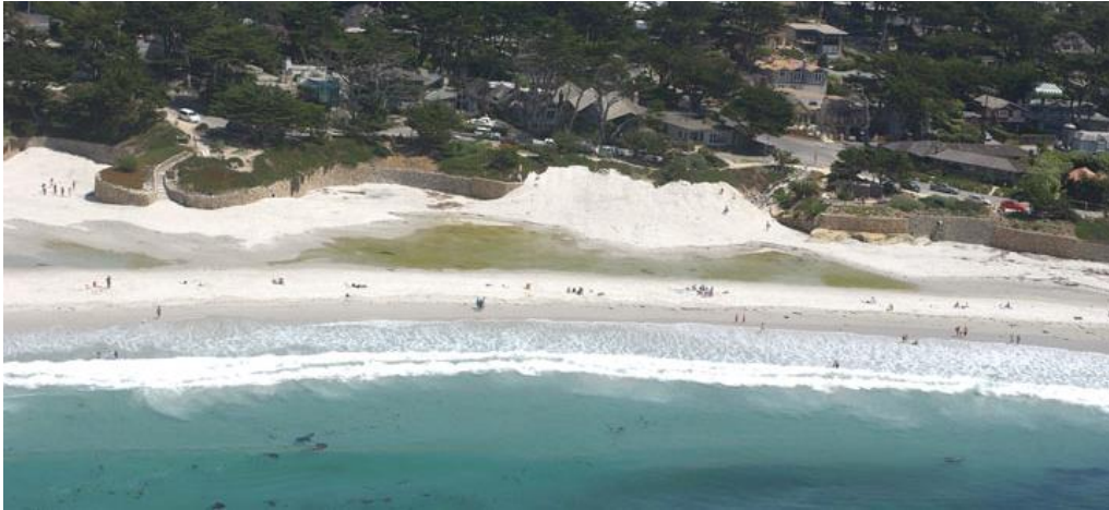
Figure 17. Beach management with sand bulldozed over the riprap revetments near 13th Avenue Source: Coastal Records Project (August 2003).
